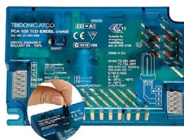
Fig. 3a: Place corridorFUNCTION plug in SMART channel and profile 2 will be used.
